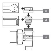
Before the soldering, the screwing and the spindle must be dismantled from the enclosure in order to avoid damages of the seals due to the heat. Do not start mounting before the casing has cooled down completely.
