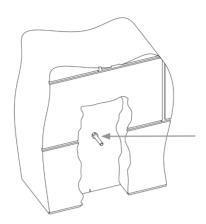
Mount the connection module and adjust the pipe elbow horizontally and at right angles to the wall.
